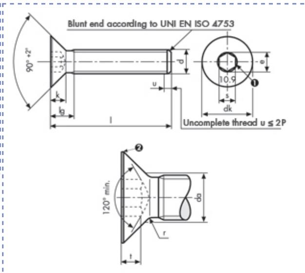
Hexagonal socket countersunk head screws
